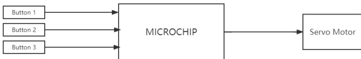
Figure 3: Block diagram of Microchip inputs and outputs
